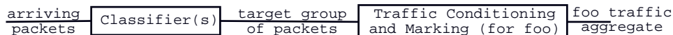
Figure 2: Relationship of the traffic aggregate associated with a PDB to arriving packets
